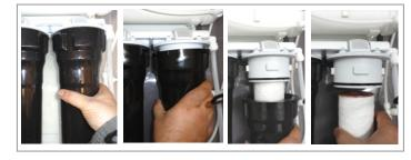
other maintenance. **NOTE:** Leave minimum of 5 inches clearance below sumps to allow removal of cartridge for replacement.
