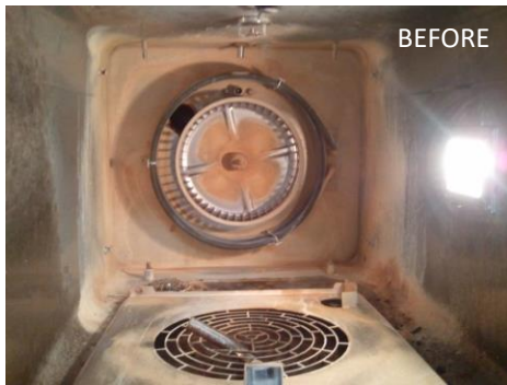
Pic (LEFT) Combi-Oven using competitive water filter system (using scale-inhibition technology) after just one week of use . Pic (RIGHT) shows the same Combi-Oven after 6 months of using Rainfresh CORO System
