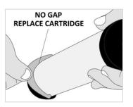
A cartridge gauge is included with the unit. After multiple cleanings, if the gauge can be passed over width of the ceramic it is time to replace the cartridge.
