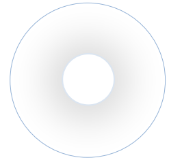
Graded Density Structure Progressively tighter towards the core for maximum dirt holding
