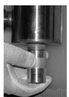
9. Carefully slide the quartz dome with top gland nut attached into the opening at the top of the UV chamber. With your other hand, use your finger to guide the dome out through the bottom opening and hold the bottom end of the quartz dome to prevent it from falling down. Hand-tighten the top gland nut into place. Do not overtighten the gland nut as it can break the quartz dome. **Note: Broken quartz domes are not under warranty.**
