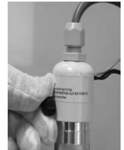
13. Remove the nut from the ground stud at the top of the unit. Next place the ground wire (green wire with yellow stripes) over the stud and tighten the nut.
